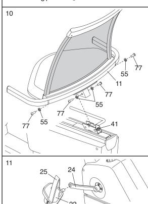
11. Identify the Left Pedal (22), which is marked with an "L." Using an adjustable wrench, firmly tighten the Left Pedal counterclockwise into the Left Crank Arm (24). Tighten the Right Pedal (not shown) clockwise into the Right Crank Arm (not shown). Important: Tighten both Pedals as firmly as possible. After using the exercise cycle for one week, retighten the Pedals.
